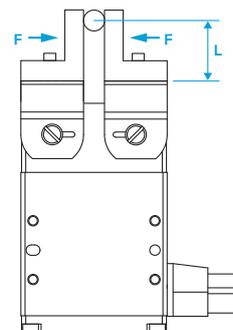
\* The gripping force of the GRLS is measured on the top face of the lever. The actual gripping force decreases in inverse proportion to the distance from the open/close fulcrum. Calculate the effective gripping force using the formula below:
